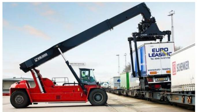
Forklifts commonly impart high wheel loads to pavements due to the cantilevered position of their loads.
